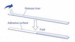
(7) Affix the side from which the release liner was removed (adhesive side down) along the front edge of the groove, leaving a 0.04" gap at the left edge of the groove.
