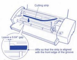
(8) Pass the right end of the cutting strip underneath the cutting head, and then move the cutting head to the left-hand side of the cutter.
